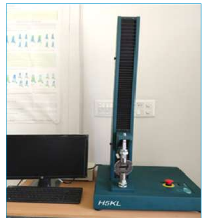
Figure 09 : 100 N Capacity UTM (Tinius Olsen).
