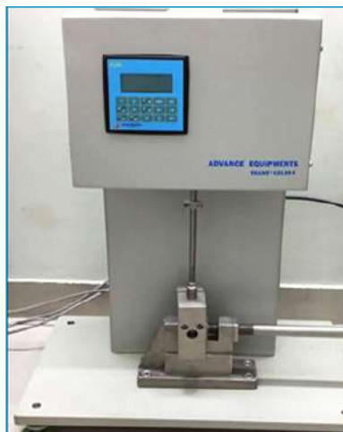
Figure 05 : Izod/Charpy computerised impact tester for polymer composites
