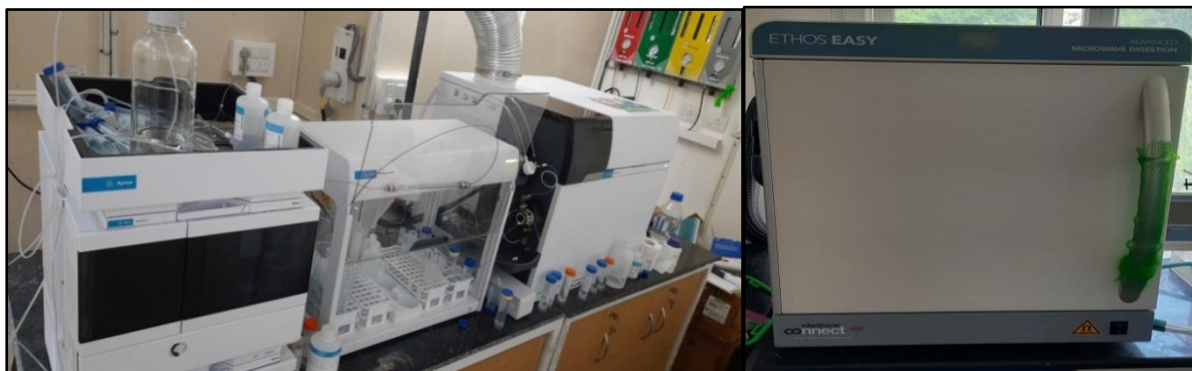
Fig: ICPMS instrument with HPLC and Microwave Digester
