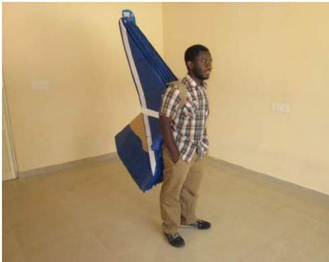
Figure 14. Full scale dome prototype in compressed form. The structure is 23cm thick and 158cm long. The entire structure weighs 15kg. Figure 15 displays how the structure gets to its collapsed form.
