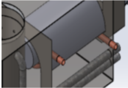
Figure 10. Copper coil to heat water while cooking
